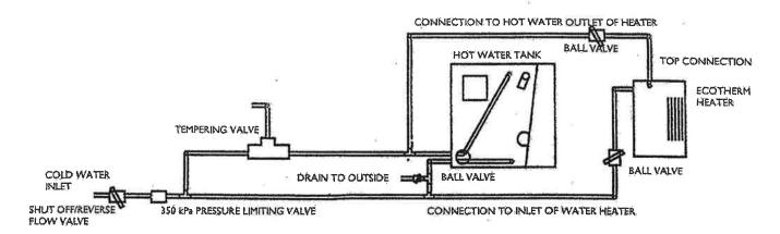
NOTE WHERE THE COLD WATER INLET IS SUPPLIED BY A PUMP FROM THE STORAGE TANK AND THERE IS AN ALTERNATIVE OUTSIDE CONNECTION FIT AN ADDITIONAL REVERSE FLOW VALVE UNLESS INCORPORATED IN THE PUMP
